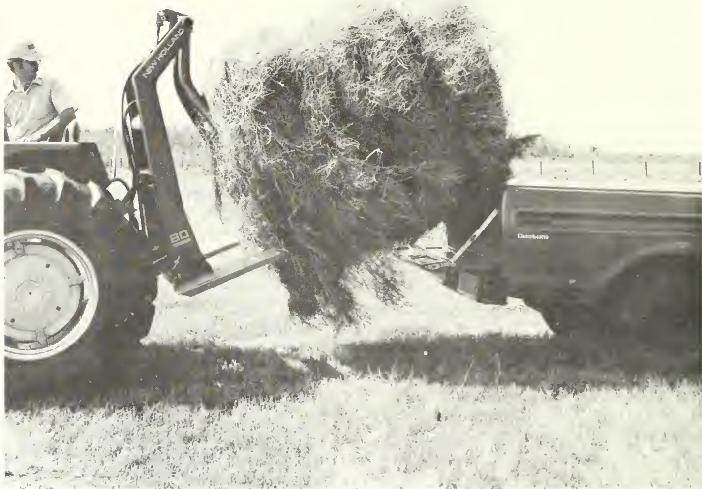
Figure 2.4.22 Rear-mounted loader with lift forks and push bar for removing round bales or other loads from forks. Courtesy: Sperry New Holland, New Holland, Pa.
