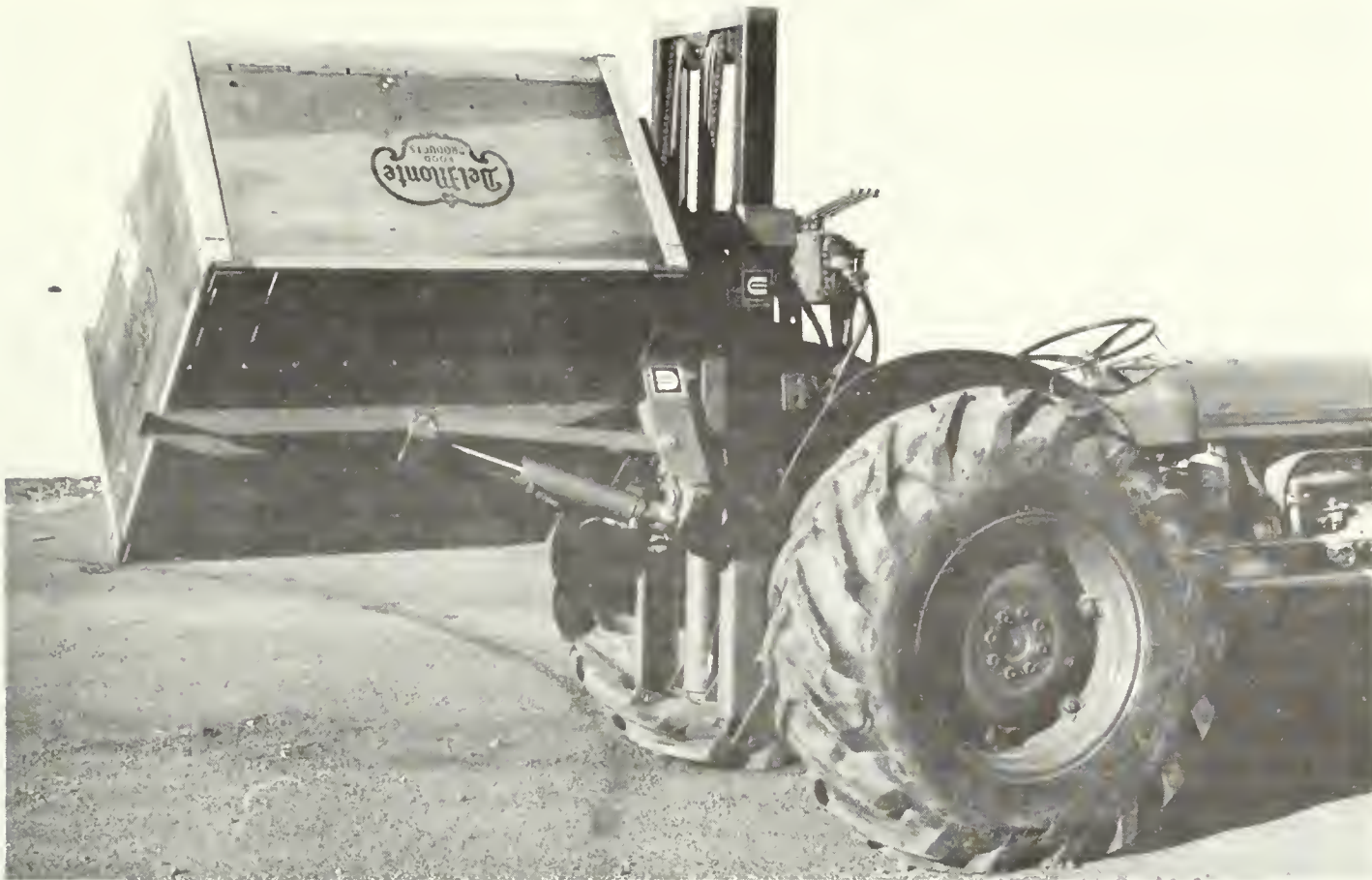
Figure 2.4.23 Hydraulic bin dumper rotates bin up to 140°. Courtesy: Edwards Equipment Co., Yakima, Wa.
