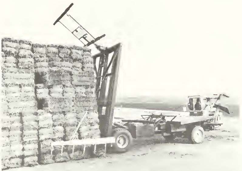
Figure 2.4.39 Self-propelled bale wagon equipped with a retriever to move entire baled hay stacks to feeding area or other stack location. Courtesy: Sperry New Holland, New Holland, Pa.
