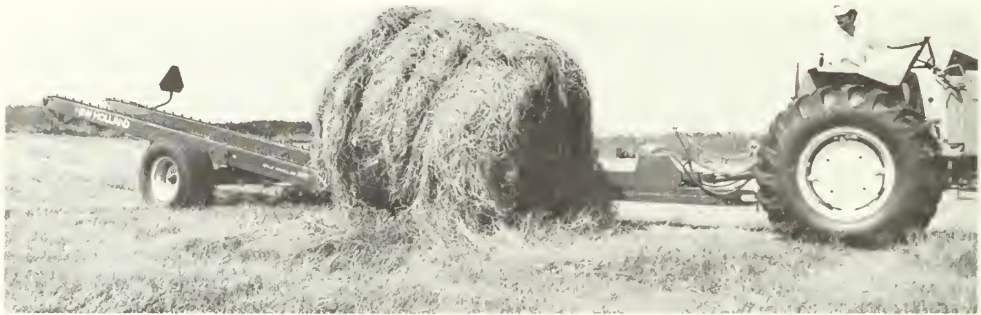
Figure 2.4.44 Tilting-bed big bale transporter with twin transfer chain. Courtesy: Sperry New Holland, New Holland, Pa.
