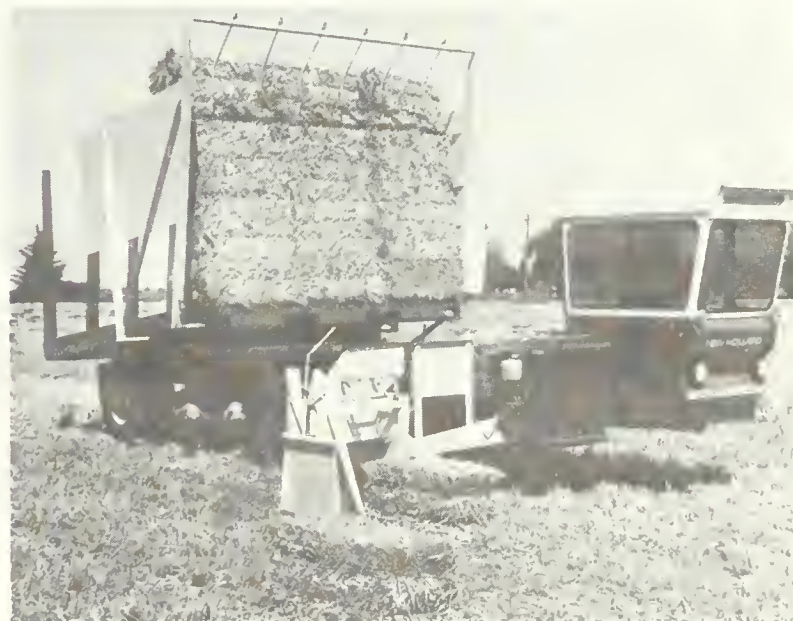
Figure 2.4.36 Automatic bale wagon can pick-up, load, transport and unload in stacks from 1.8 to 5.5 t (2 to 6 tons) per load. Courtesy: Sperry New Holland, New Holland, Pa.
