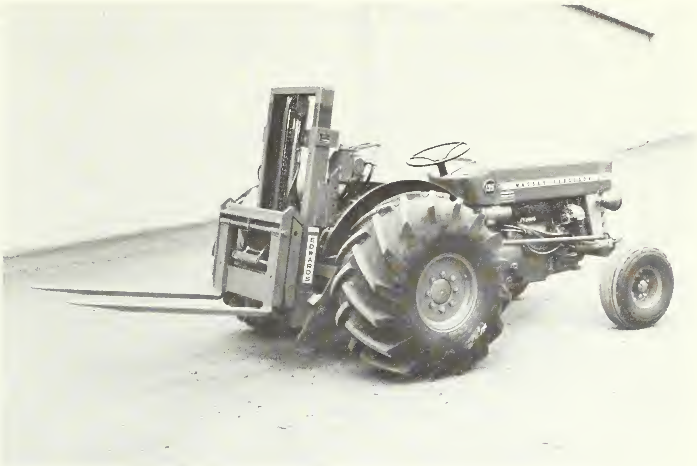
Figure 2.4.15 Rear-mounted bin stacker, 1 tonne capacity, lift heights available from 1m to 2.7m. Courtesy: Edwards Equipment Co., Yakima, Wa.
