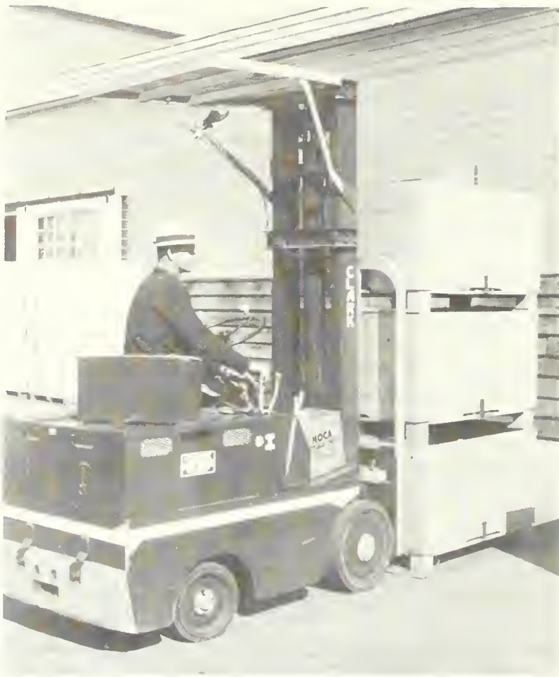
Figure 2.4.13 Electric fork lift. Useful for loading, unloading, transporting and stacking bins in a packing house.
