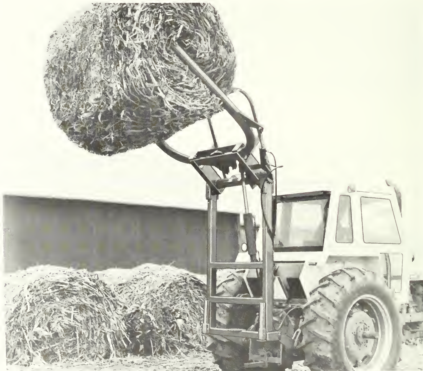
Figure 2.4.45 Tractor rear-mounted single bale pick-up attachment. Can be used for stacking and unrolling for cattle feeding. Courtesy: Gehl Company, West Bend, WI.
