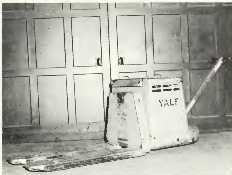
Figure 2.4.11 Low-lift pallet lift. Useful for moving one to two bins in a packing house.
