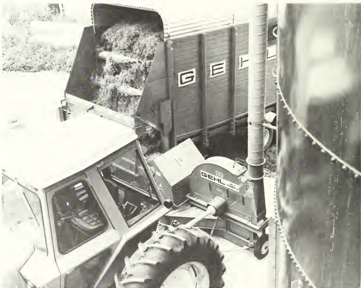
Figure 2.4.31 Self unloading wagon supplies chopped forage to forage blower. Courtesy: Gehl Co., West Bend, Wisconsin.
