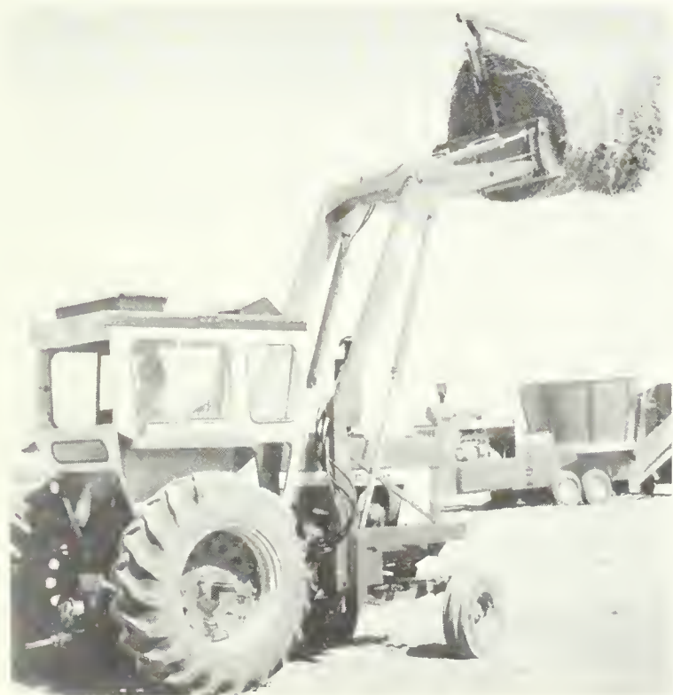
Figure 2.4.42 Big bale fork attachment for front-end tractor loader will handle 1.5 to 2.1 m bales. Courtesy: Farmhand Inc., Hopkins, Minn.
