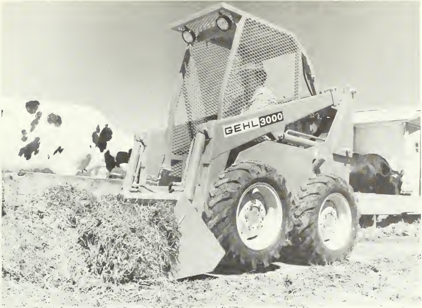
Figure 2.4.20 Skid-steer loader for front-mounted bucket, fork or blade. Courtesy: Gehl Company, West Bend, WI.
