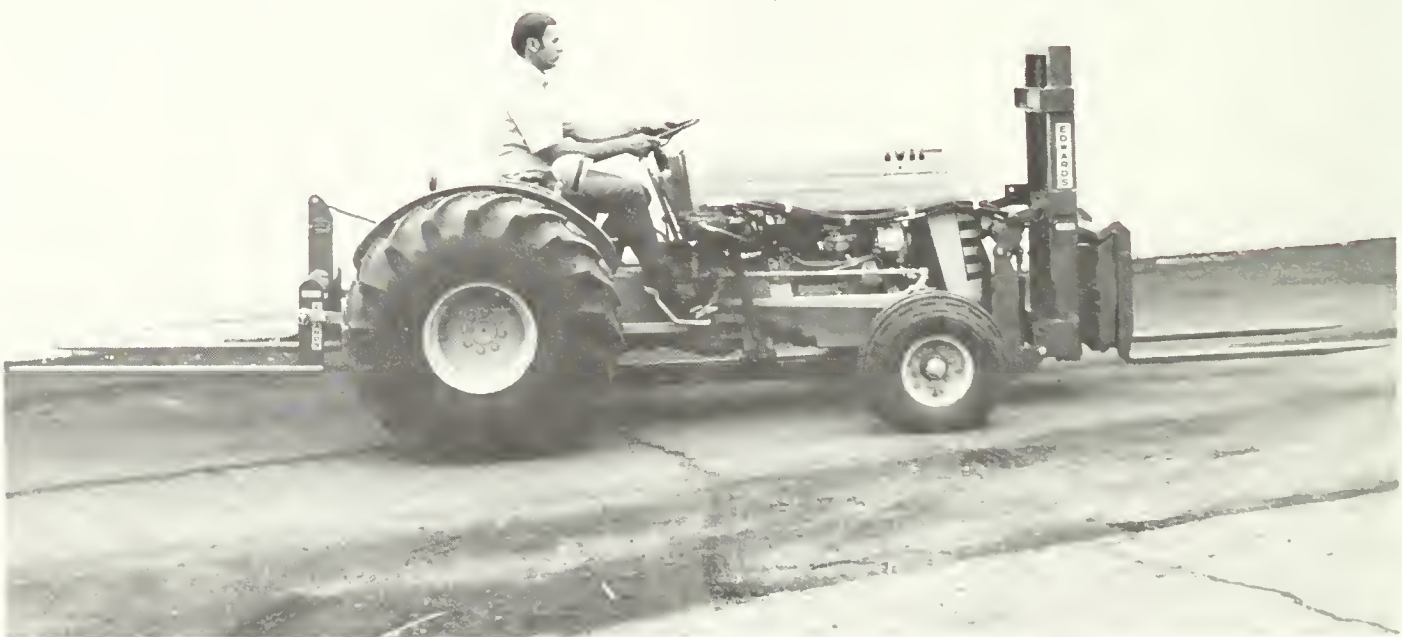
Figure 2.4.14 Front-mounted bin stacker and rear-mounted three-point hitch transporter for tree to tree handling of bins. Rear-mounted unit lifts 0.7t up to 0.4 m. Courtesy: Edwards Equipment Co., Yakima, Wa.
