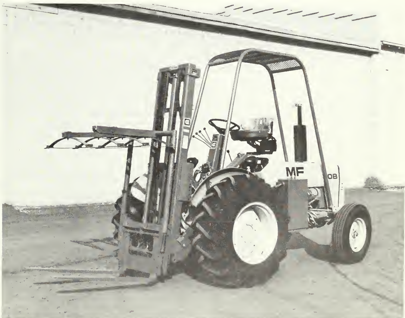
Figure 2.4.16 Hydraulic rear-mounted fork lift with hold down attachment. Will lift 1.8 t from 1.5 to 3.6 m. Courtesy: Edwards Equipment Co., Yakima, Wa.
