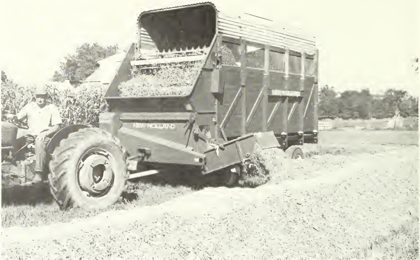
Figure 2.4.30 PTO powered chain and slat self unloading wagon. Courtesy: Sperry New Holland, New Holland, Pa.
